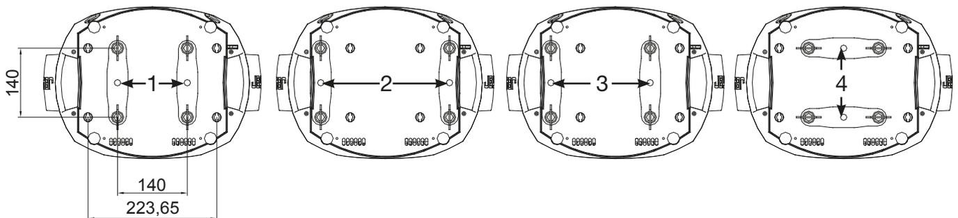
The Camlocs must snap in to be locked properly. Ensure that the structure (for example a truss system) to which you are attaching the fixture is secure. If you install the fixture to a hanging system (for example to a truss system) always attach a safety cable, that can hold at least 10 times the weight of the fixture. There is a corresponding eyelet on the fixture for the secondary safety device (see picture).
