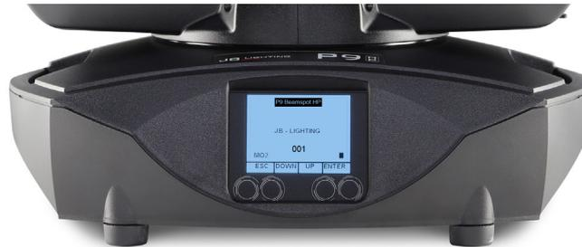
Special areas can only be called up using a specific key combination. To do this, press and hold the "ENTER" key and then use the opposite "ESC" key to access the menu. To exit the function, proceed in reverse order.
