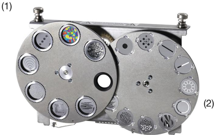
To change the rotating gobos remove only the clamping ring (A) with a pointed object replace the gobo and then put the clamping ring again. When installing glass gobos, make sure the white coated side faces the front lens. Gobos that are not allowed to twist, e.g. Logos are additionally recommended to be secured against twisting with a drop of silicone adhesive.
