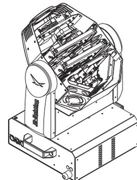
If changing the lamp, remove old lamp from lamp socket. Hold the new lamp only by its ceramic base. Never touch the glass bulb.
