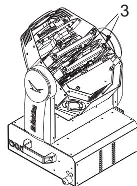
The gobos are fixed by means of a spring. To change gobo remove spring and gobo and insert the new gobo. Readjust the spring to fix the gobo. Make sure that the blacked side of the metal gobo is positioned opposite the lamp (in direction of the objective). If you insert glass gobos make sure that the coated side is positioned in opposite direction to the lamp.
